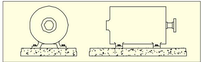
Figure 2. Electric motor that had a resonance at  $2 \times$  running speed  $\sim 7100$  CPM. The entire motor vibrates as a single mass.
