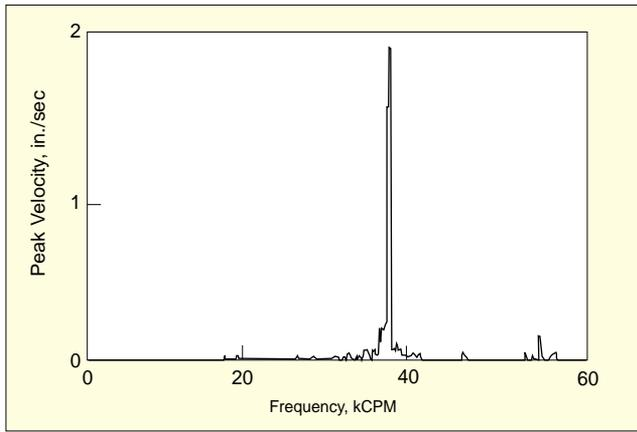
Figure 4. Vibration spectrum of the input bearing in the axial orientation. Note the very high level of vibration at approximately 36,000 CPM. This frequency corresponds to the gear meshing frequency.
