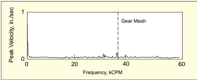
Figure 7. Vibration spectrum of the gearbox after installing the inertial mass and running for approximately one week. Compare the amplitude of vibration at the fugitive frequency in this spectra with that in Figure 4. The amplitude scales in both Figures 4 and 7 are the same, and both surveys were conducted under similar operating conditions.
