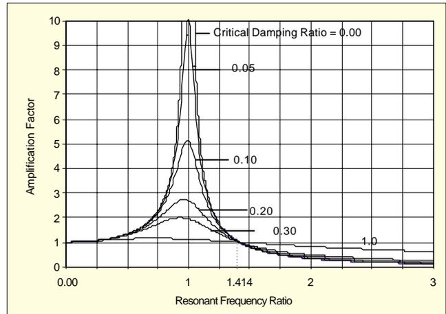
Figure 1. Amplification factor versus resonant frequency ratio for several critical damping factors.
