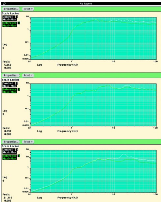
Figure 15. Reference Response Spectra (RRS) and Control Maxi-Max SRS for X, Y and Z axes.
