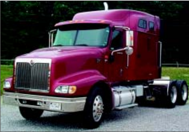
Figure 1. International® 9400i Class-8 tractor with the High-Rise Pro Sleeper®. Integrated-sleeper height of 196 cm by 183 cm deep.
