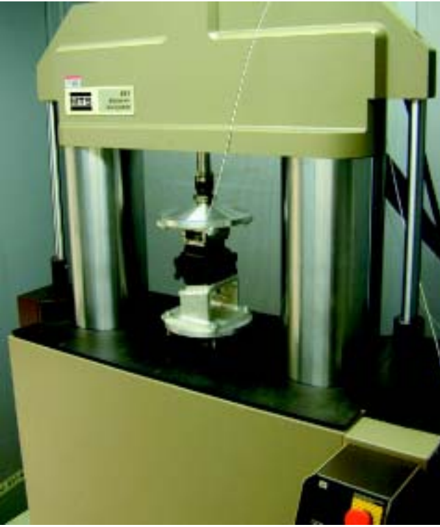
Figure 5. MTS elastomer testing system being used to evaluate the dynamic characteristics of a hydraulic engine mount.
