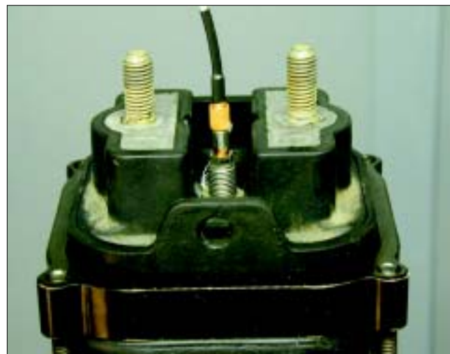
Figure 4. Dynamic pressure transducer installed in the top chamber of a hydraulic engine mount.
