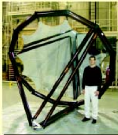
e) 3-m hexapod reflector for active control experiments (projected dots on stretched membrane reflector)
