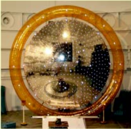
a) 5-m inflatable parabolic reflector
