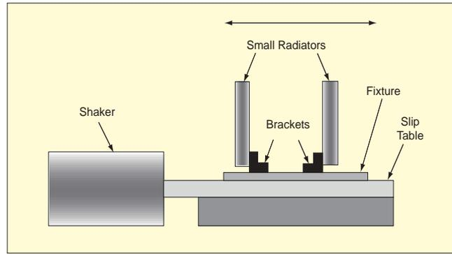
Figure 5. Test setup in the "slip-table" mode.
