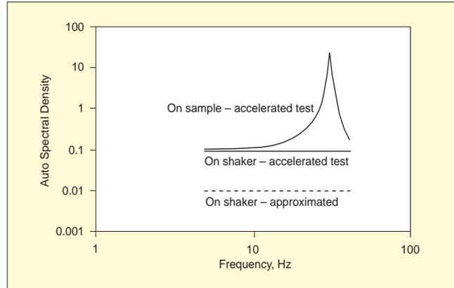
Figure 6. The auto spectral density  $g^2/\text{Hz}$  of the acceleration of the shaker and sample.
