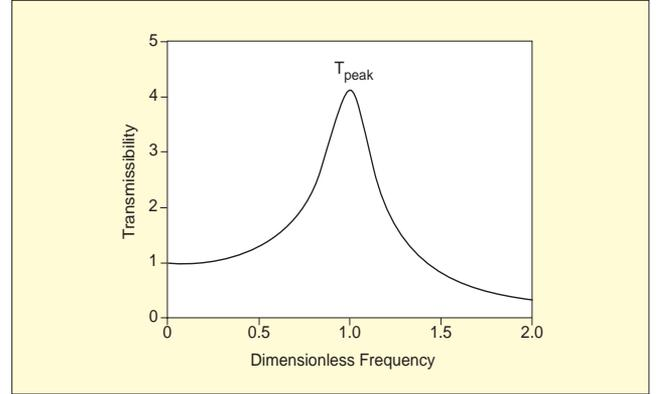
Figure 4. The transmissibility of the 1-DOF vibration system from Figure 2. The dimensionless frequency equals  $f/f_r$ .
