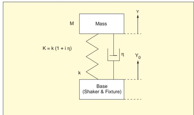
Figure 2. Single-degree-of-freedom vibration system. The damping element is a dashpot but in Equation (2), a more general case of damping is considered.
