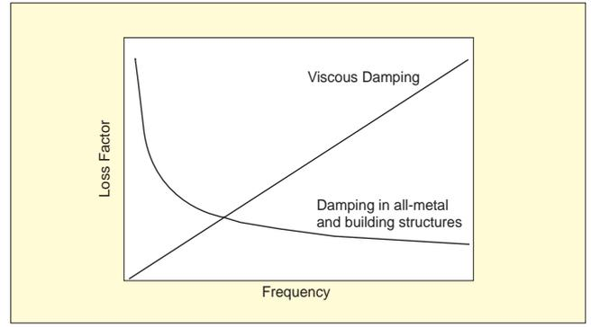
Figure 3. The loss factor dependence on frequency for two different damping mechanisms.
