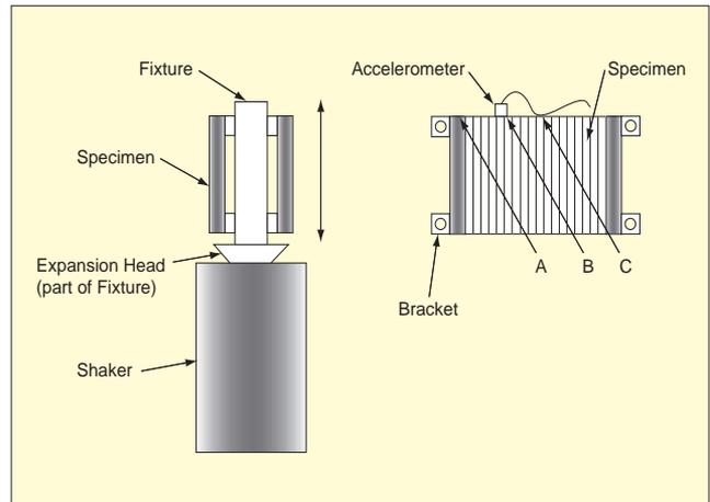
Figure 1. Test setup for 1-DOF shaker test on two condensers symmetrically installed on the fixture.
