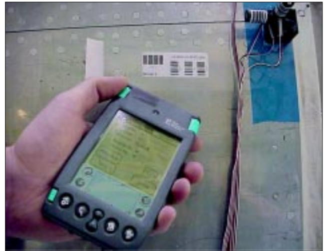
Figure 5. Barcode scanning using a hand held personal digital assistant verifies transducer installation and provides data for easy merging with test configuration files.
