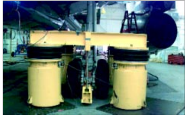
Figure 6. Soft support (shown under right main landing gear), floats airplane inches from floor.
