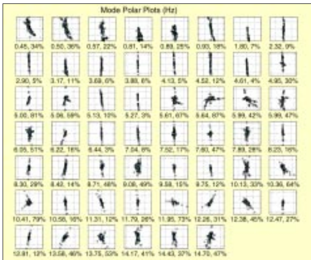
Figure 23. Polar plots of test modes reveal complexity and 'noise' on some modes.
