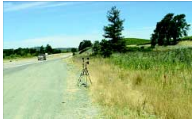
Figure 7. Microphone at 7 m, looking north (diamond grind Site 2).
