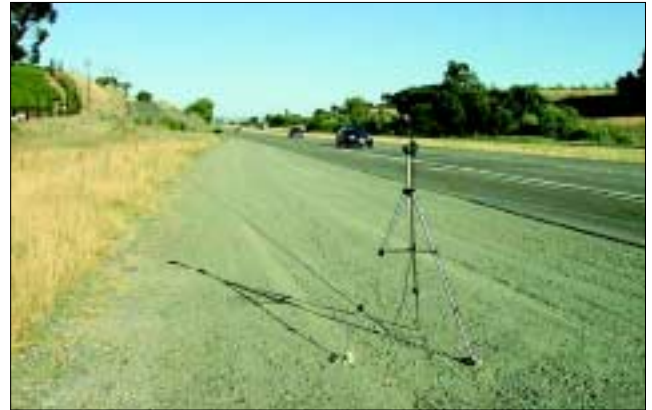
Figure 6. Microphone at 7 m, looking south (diamond grind Site 2).
