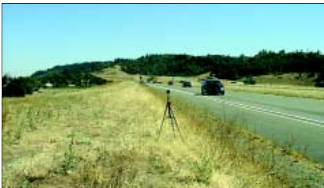
Figure 5. Microphone at 7 m (grooved Site 1).
