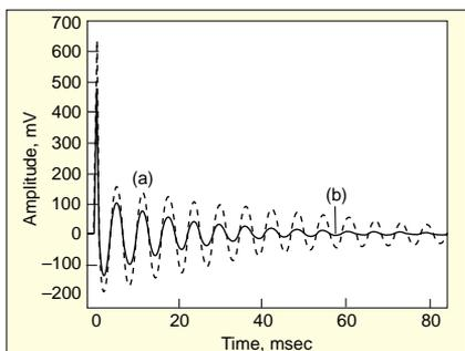
Figure 6. Time responses: (a) with Rectangular window; (b) with Exponential window.
