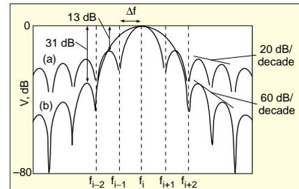
Figure 2. Comparison of spectra for the Rectangular window (a) and the Hanning window (b).
