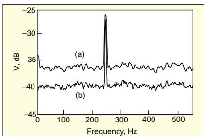
Figure 4. Comparison of spectra of a sine wave buried in random noise with: (a) the Flat-Top window; and (b) the Hanning window.
