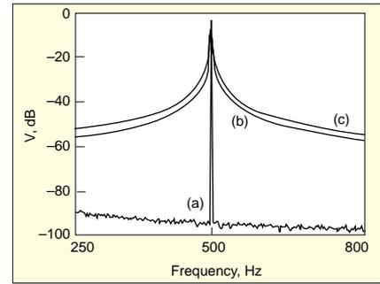
Figure 1. Spectrum of a sine wave with the Rectangular window: (a)  $f = f_0$ ; (b)  $f = f_0 - \Delta f/8$ ; (c)  $f = f_0 - \Delta f/2$ .
