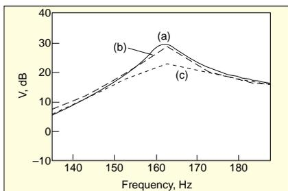
Figure 5. Transfer functions: (a) baseline; (b) with Rectangular window; (c) with Exponential window.
