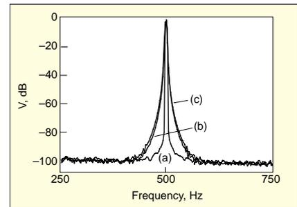
Figure 3. Spectrum of a sine wave with the Hanning window: (a)  $f = f_0$ ; (b)  $f = f_0 - \Delta f/8$ ; (c)  $f = f_0 - \Delta f/2$ .
