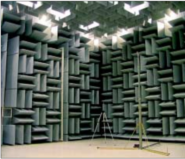
Figure 5. Inside the hemi-anechoic chamber.
