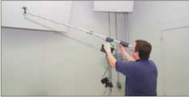
Figure 14. Rotating microphone setup inside the reverberation chamber.
