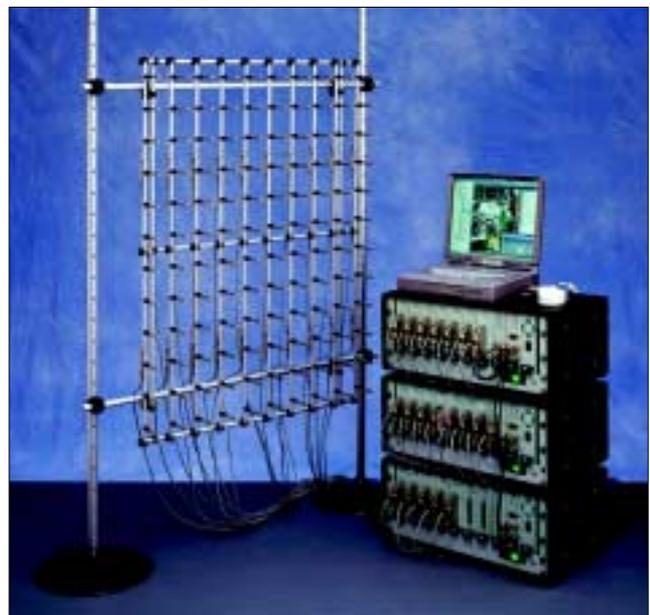
Figure 17. NS-STSF technique, full-sized microphone array.
