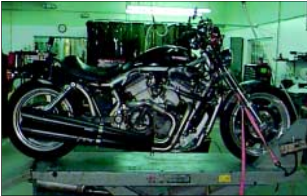
Figure 2. Early development exhaust system on VR1000 powered "test buck."
