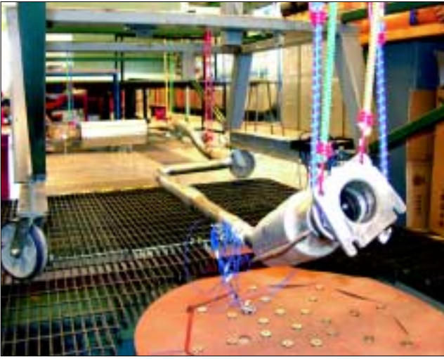
Figure 4. Photo of exhaust subsystem under investigation supported with elastic cords to approximate free-free boundary conditions.
