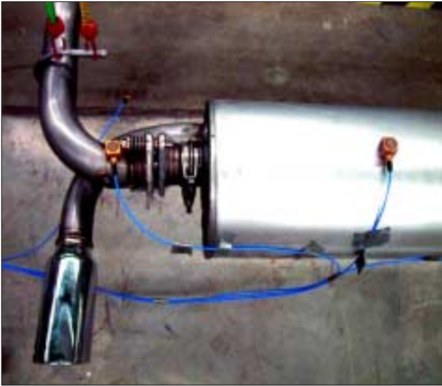
Figure 10. Photo of inlet pipe of muffler fitted with Metex joint for reducing the exhaust torsional coupling stiffness at that location to mitigate the vibration problem.
