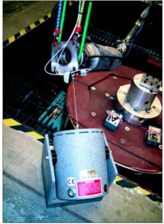
Figure 6. Electrodynamic shaker attached with stinger to front bracket of exhaust system in front of the bellows to simulate input from powertrain.
