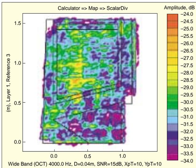
Figure 8. Side door transmission loss close to the glazing coincidence frequency (4 kHz).
