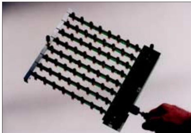
Figure 1. 64-channel microphone array.
