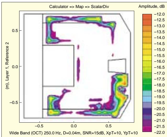
Figure 4. Floor transmission loss at 250 Hz showing direct noise path through air vents and steering pedals.
