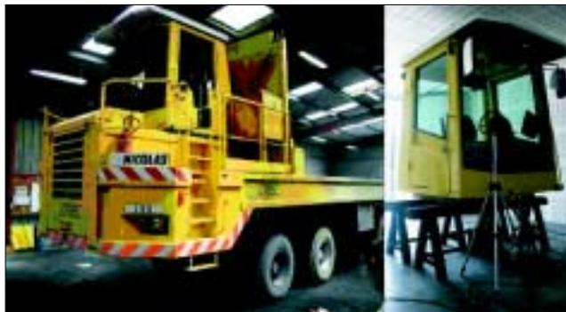
Figure 2. Cab mounted on the truck and in the test cell.
