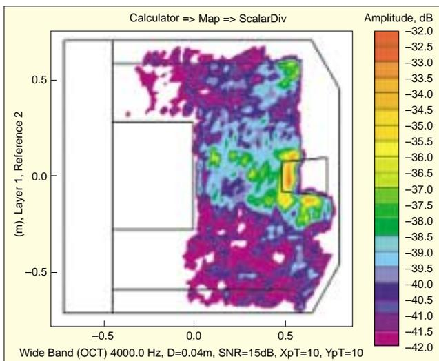
Figure 5. Floor transmission loss at 4 kHz showing leaks around the steering rod.
