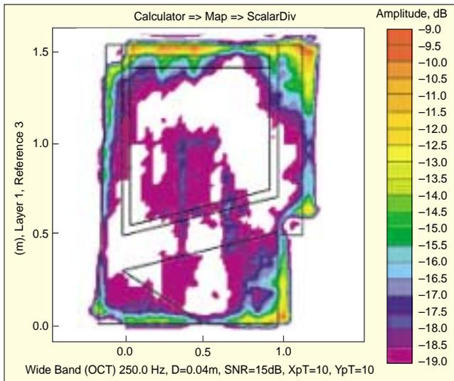
Figure 7. Map of the side door at 250 Hz showing a transmission loss defect along the door seal.
