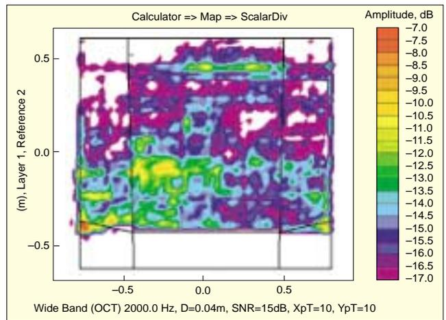
Figure 6. Map of the front windshield transmission loss at 2 kHz. A defect is identified at the lower left corner coming from poor sealing efficiency.
