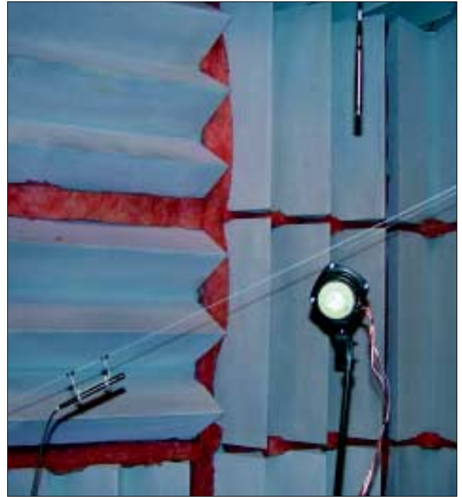
Figure 2. Traverse line and microphone, source and stationary reference microphone (located above source).
