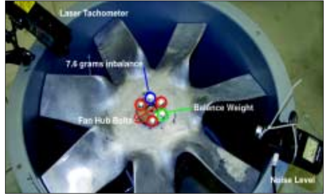
Figure 3. Fan with imbalance weight.
