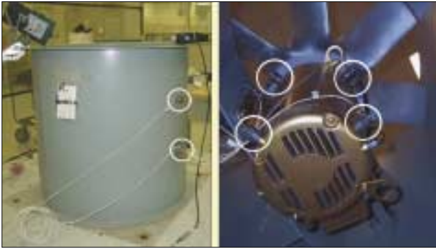
Figure 1. Fan cowling vibration transducers (left) and motor bearing housing transducers (right).
