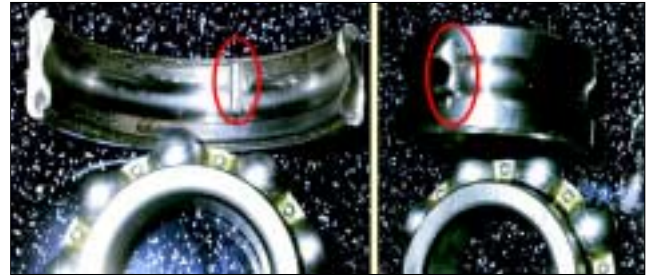
Figure 2. SKF® 6503 and 6502 deep groove bearings with race defects.
