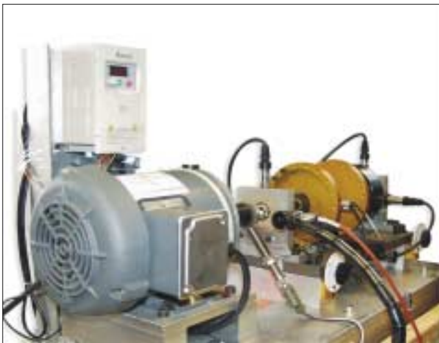
Figure 1. Top - The PXI-based data acquisition system contains 24 channels of 24-bit dynamic signal acquisition, multiple temperature, pressure, and tachometer inputs, and a 6 1/2 digit DMM. Bottom - A 4-pole motor drives the unit under test, a seven-blade cooling fan.
