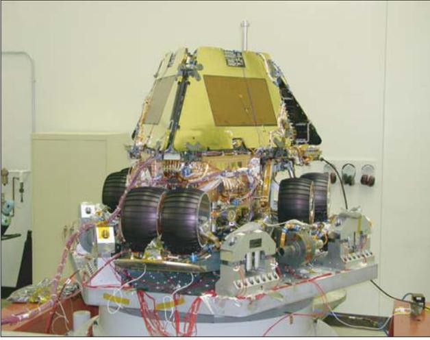
Figure 1. Shock testing on an electrodynamic shaker. Mars Exploration Rover #1 undergoing vertical axis landing loads pulse testing at JPL on an LDS Model 994 shaker. Photo courtesy of the Jet Propulsion Laboratory, California Institute of Technology.
