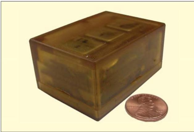
Figure 1. MicroTAU: Micro Triaxial Accelerometer Unit.
