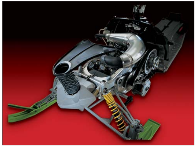
Figure 3. Forced air induction system.
