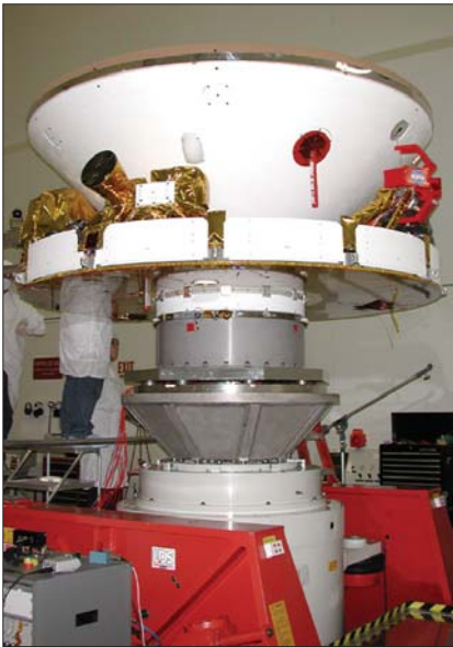
Figure 3. One of two Mars Exploration Rovers sits inside its Cruise stage waiting to undergo vibration testing at NASA'S Jet Propulsion Laboratory. The LDS V994 is the largest shaker system in the world and can produce 65,000 lbs peak force.
