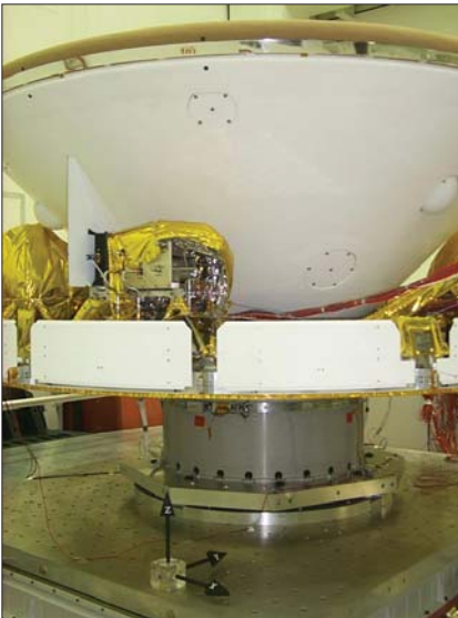
Figure 4. The Mars Rover mounted on the slip table for the LDS V994 Shaker. The multiple hydrostatic bearings restrained overturning moments associated with the lateral vibration of the Rover.
