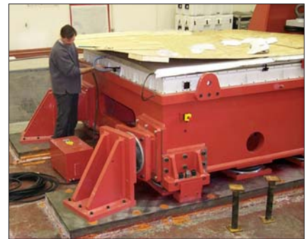
Figure 2. Slip table assembly for V994 Shaker showing additional lateral restraint assembly.
