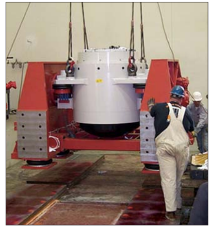
Figure 1. The LDS V994 Shaker being positioned in the JPL Dynamics Test Laboratory.
