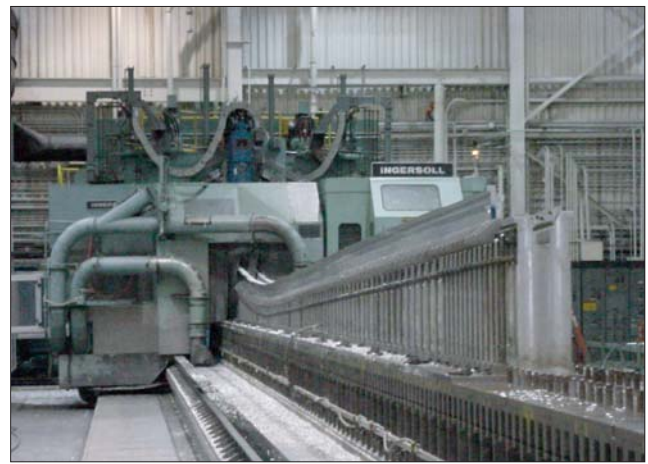
Figure 3. Milling machine with aluminum extrusion clamped on top of fixturing.
