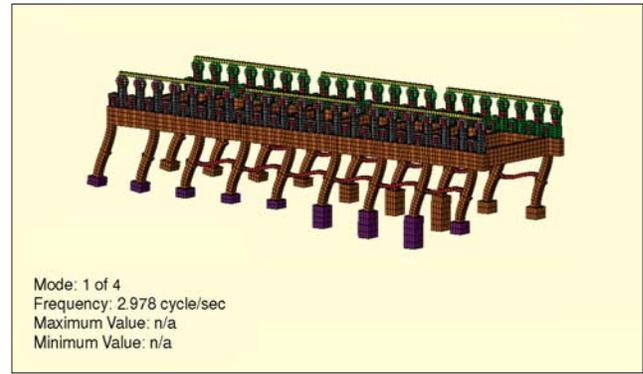
Figure 9. Mode shape of paper machine.
