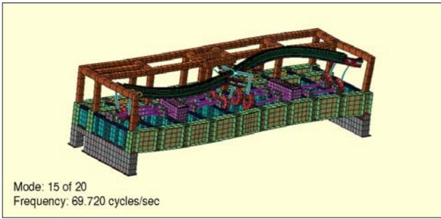
Figure 7. Mode shape of proprietary machine.
