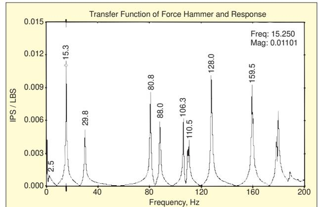
Figure 10. Impact test results for fan.
