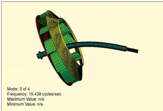
Figure 11. FEA results for fan rotor.
