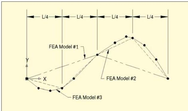
Figure 2. FEA results for beam mode shape.
