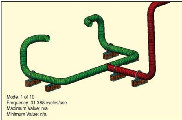
Figure 3. FEA model of piping systems.
