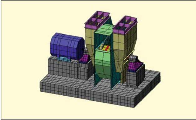
Figure 8. FEA model of fan foundation.
