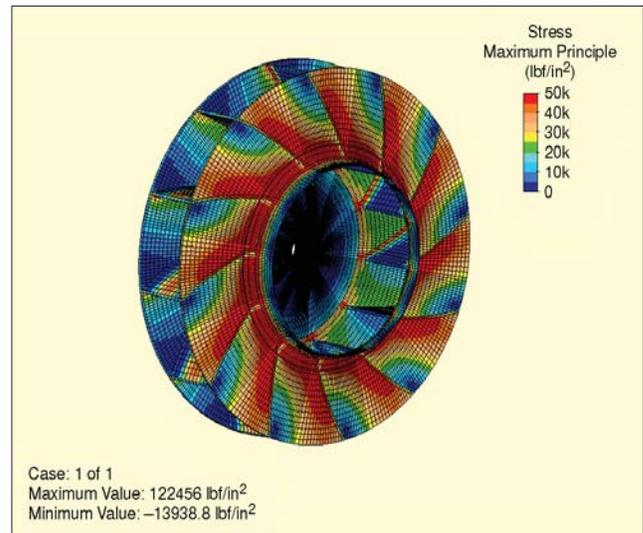
Figure 12. Centrifugal stress in fan wheel.
