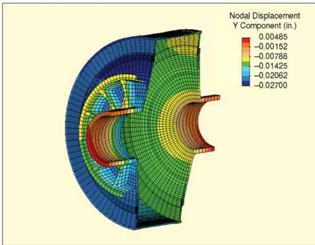
Figure 1. FEA model of grinding mill.
