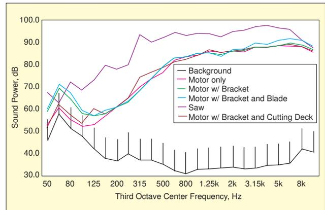
Figure 5. Sound power contribution of various sources within the saw.
