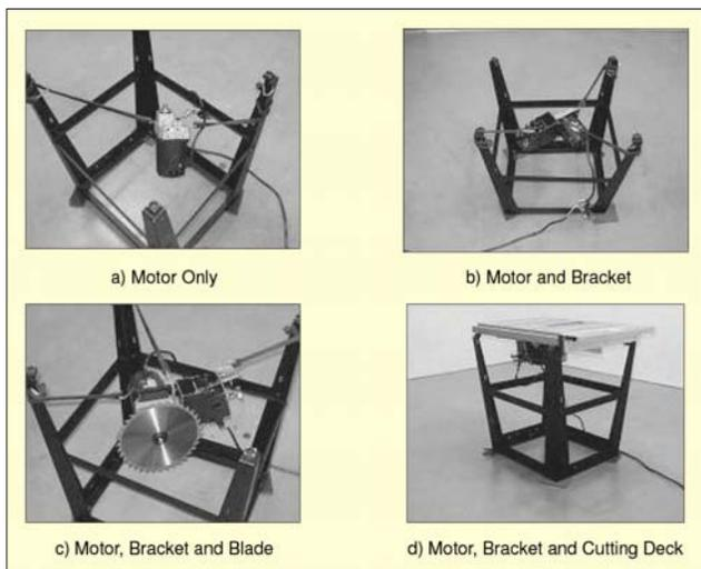
Figure 1. Test setup configurations for component sound power measurements.
