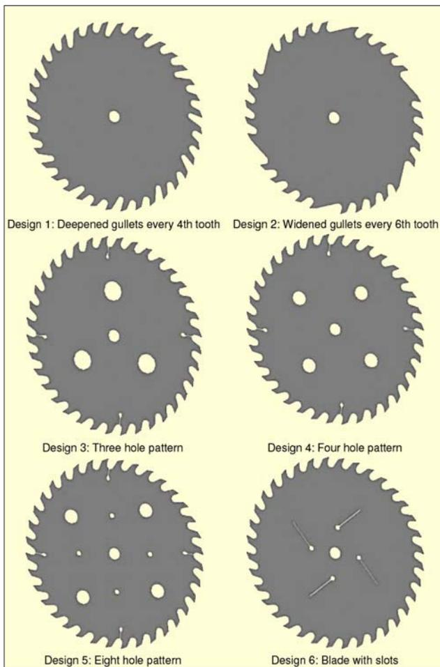
Figure 13. Modified saw blade designs.
