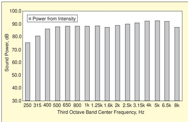
Figure 7. Sound power levels from sound intensity measurements.
