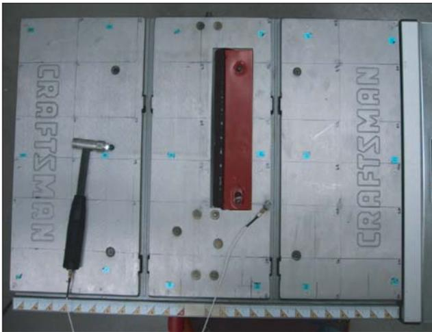
Figure 4. Setup for cutting deck modal analysis.
