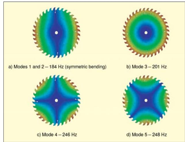
Figure 9. Original saw blade mode shapes for modes 1-5.
