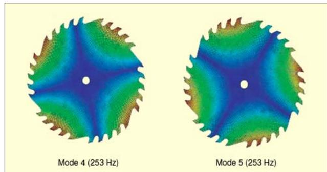
Figure 15. Wide gullet (every 6th tooth) blade – mode shapes 4 and 5.
