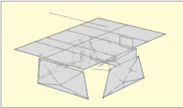
Figure 3. Geometry of the table saw for ODS test.
