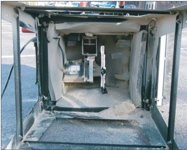
Figure 11. Acoustical foam treatment for chassis interior.
