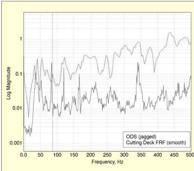
Figure 8. Comparisons of ODS vs. cutting deck modal analysis data.
