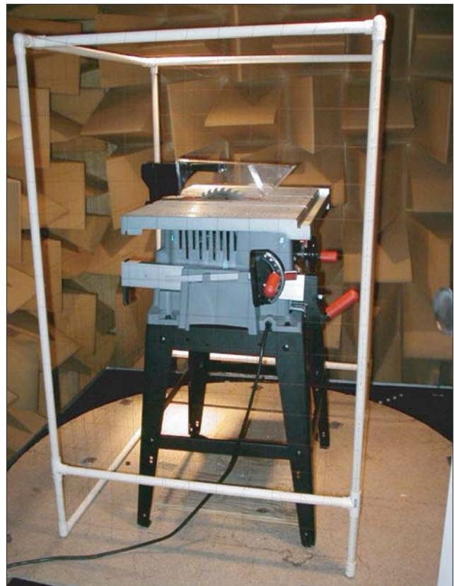
Figure 2. Setup for point-by-point sound intensity test in the anechoic chamber.
