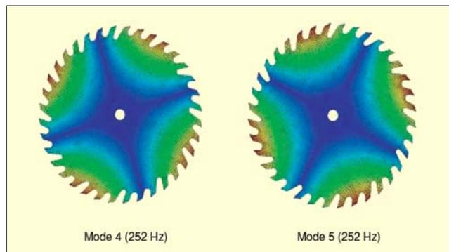
Figure 14. Deep gullet (every 4th tooth) blade – mode shapes 4 and 5.
