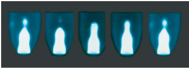
Figure 6. Sequence of frames from a slow motion movie of the oscillating flame. Note – The frames show the flame size at instances 1/4 of a cycle apart. The last frame shown is a repeat of the first.
