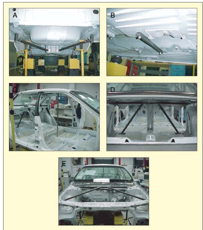
Figure 3. A - quad box to rail support, B - tunnel strap, C - floor to roof pole, D - rear shocks to rear floor support, E - front shock to radiator support.
