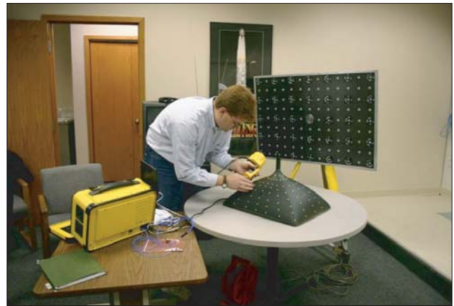
Figure 12. Total data acquisition time on the TV tube with the digitizer was 10 minutes.
