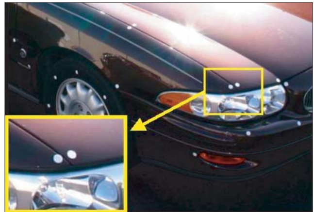
Figure 5. 3/4 in. circular targets placed on car.
