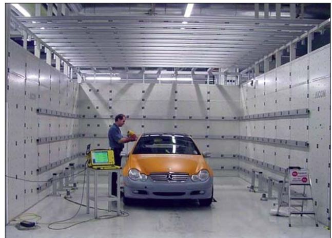
Figure 13. Calibrated rooms eliminate the need for temporary panel positioning.
