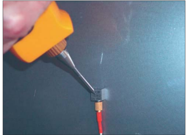
Figure 4. TEDS sensor with precision machined locator holes for digitizing 6 DOF coordinates.
