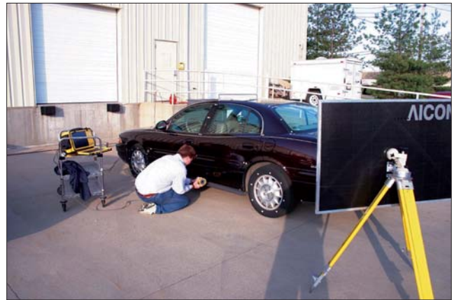
Figure 8. Using the photogrammetric digitizer to collect geometry on an automobile.
