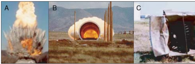
Figure 1. Examples of freely expanding (A), directed (B), and contained air-blasts (C).
