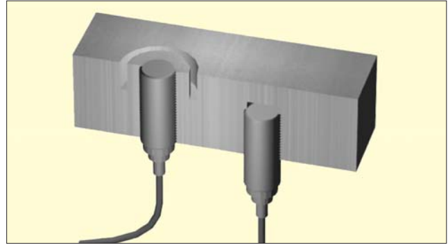
Figure 11. Strain isolated pressure transducer left – isolated 'check' transducer right.
