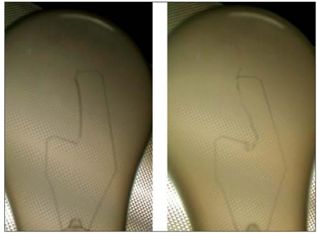
New 75-watt "Do-It" light bulb before test (left) and after test (right) with a Gaussian ( $k = 3$ ) random vibration excitation for 54 minutes.
