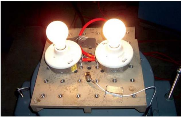
Figure 9. Setup for vibration testing of light bulbs with kurtosis.
