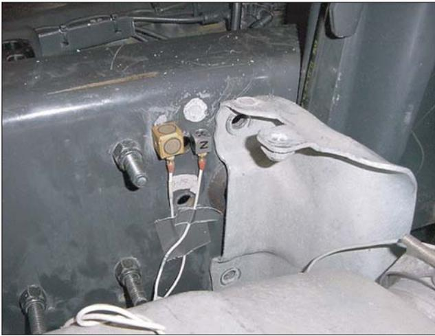
Figure 8. Accelerometers attached to the engine mount position and the exhaust system attachment point respectively, illustrating the close proximity.
