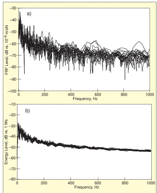
Figure 2. a) Variation of FRF levels between points on two subsystems, calculated for an L-plate ensemble. b) Variation of spatial average velocity level in the receiving plate of the L-plate ensemble. Combined local parameter variation standard deviations: 2% for eigen frequencies and 20% for the logarithm of modal damping.<sup>7</sup>
