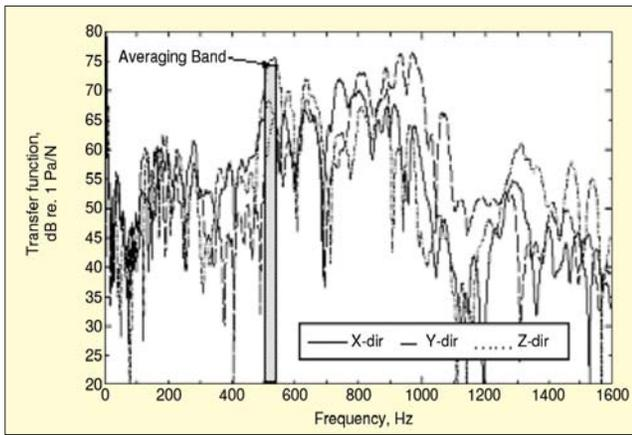
Figure 5. Example of measured noise-to-force transfer functions (dB re. 1 Pa/N). A typical frequency averaging band is illustrated.
