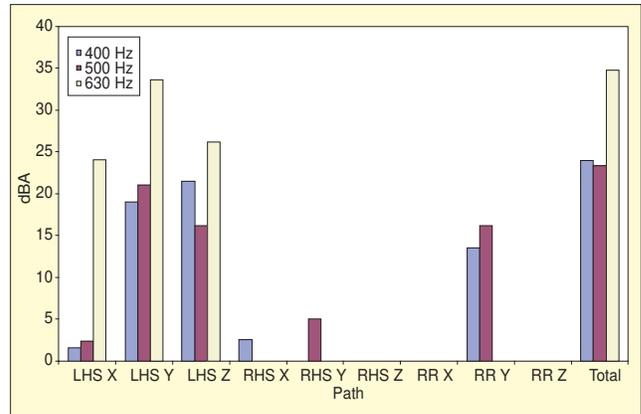
Figure 7. Ranking of transfer paths for structure borne gear whine (1st gear, slow speed)
