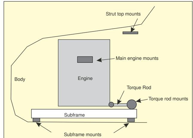
Figure 3. Sketch of the engine installation for the idle noise and vibration case. The wheel suspension has McPherson struts with lower wish-bone link arms that are attached to the subframe.
