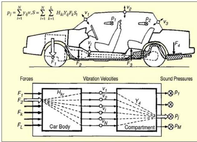
Figure 1. The principle of transfer path analysis.
