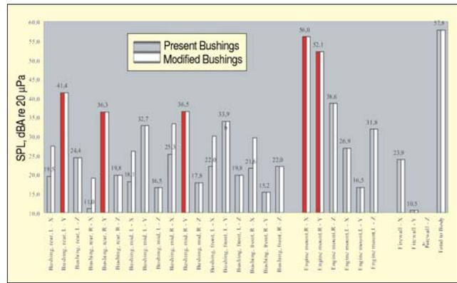
Figure 6. Example of transfer path ranking for one pump blade order at a specific speed.
