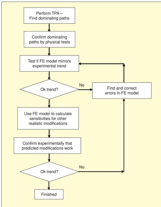
Figure 4. The process of using TPA and CAE to find solution to an idle NVH problem late in a new car development. The philosophy may be used in other similar situations.
