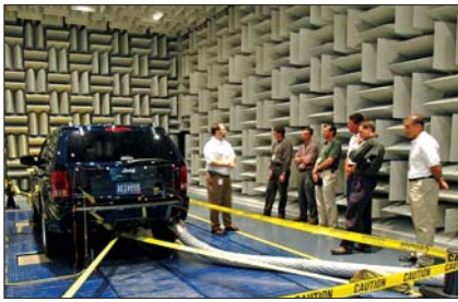
ARC's 4WD Link dynamometer is designed to simulate vehicle operating conditions in a hemi-anechoic test chamber.
