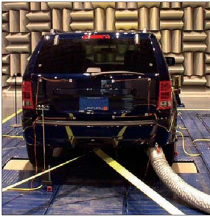
Figure 3. Model 4900 chassis dynamometer at ARC facility.
