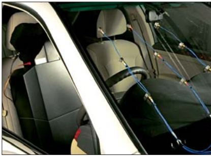
Figure 2. Sensors measure interior noise.
