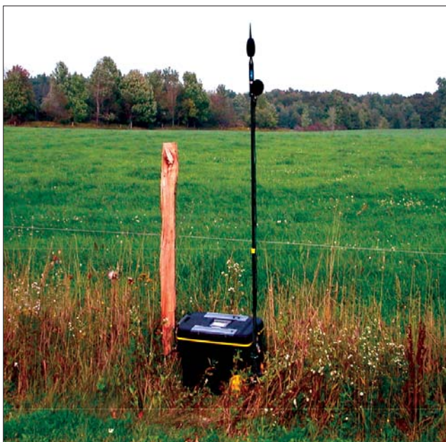
Figure 7. Portable sound monitoring system containing a standard Type 1 sound level meter and additional meter with digital audio recording capability.
