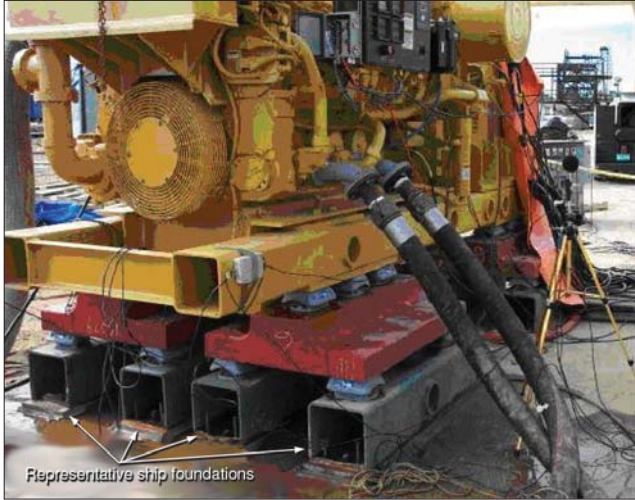
Figure 4. Factory test of genset installation.
