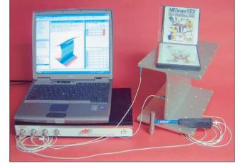
ME'ScopeVES uses Vibration Research 8500 shaker-controller to acquire impact data.
