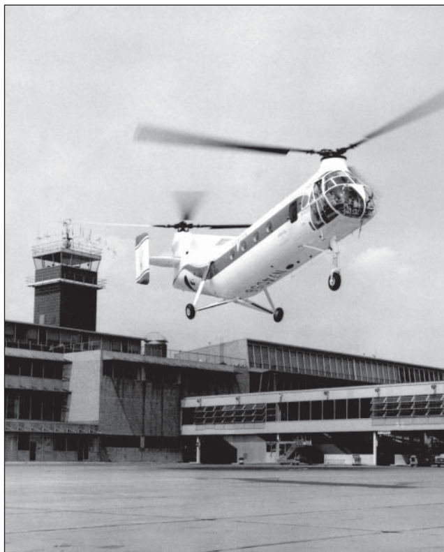
A short time after our noise measurement program was completed, Piasecki became Vertol, and the military H-21 was modified to become the Vertol Commercial Model 44 Helicopter (shown here), which received our recommended acoustic treatments. With an enclosure around the overhead drive shaft and some well-designed interior lining for the cabin walls, we achieved a noise reduction of about 5 decibels in the low frequency region (where the vibration was dominant) and 22 to 26 decibels in the speech frequency octave bands.
