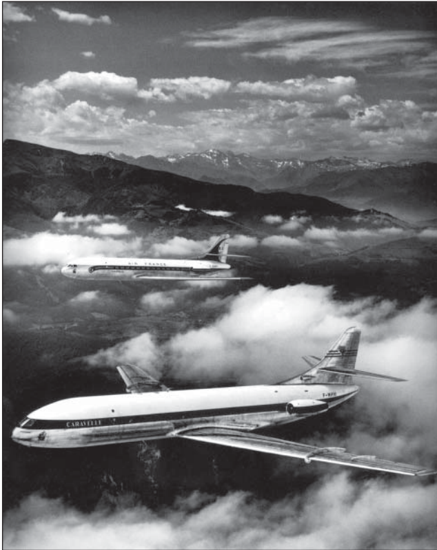
Twin-engine "Caravelle" jet airliner produced by Sud Aviation of France. This was the first of the commercial jets to meet the noise requirements of the Port of New York Authority. Takeoffs and landings of the Caravelle were measured by Leo Beranek and Laymon Miller at Orly Airport, Paris, in 1957.
