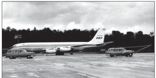
At Boeing Field in Seattle in 1958. Two vehicles with sound recording equipment circle the new production-model Boeing 707 with its engines at takeoff power, to obtain data for determining the sound power level of the aircraft. Note the microphone at the end of a boom out in front of each car so as to minimize any distortion of the sound field.
