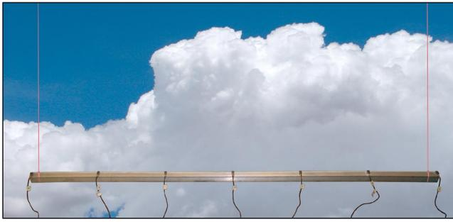
Figure 3. Photo of lightly damped aluminum beam with variable-length elastic supports.
