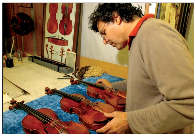
Figure 2. Even three-century-old violins require critical attention to string choice, soundpost placement and bridge adjustments (the bridge is one of two major energy filters on the violin) to maintain quality. Here renowned violinmaker Sam Zygmuntowicz checks the three old Italian violins to ensure that they are at peak performance.
