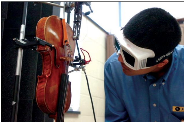
Figure 4. Vikrant Palan of Polytec sets an alignment point to aid in splicing top, back, and rib scans into a three-dimensional model with proper orientations.
