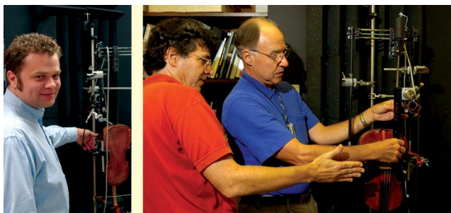
Figure 3. Danial Rowe (left), one of the official “hammer twangers,” manually cocking-fires force hammer on a Stradivari violin. Sam Zygmuntowicz (red shirt) and George Bissinger adjust force hammer position.
