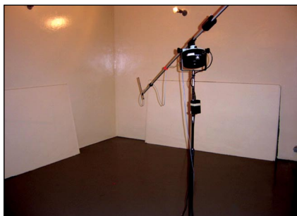
Figure 1. The microphone at end of boom arm moves continuously up, down, left, and right as dozens of successive tests are run.
