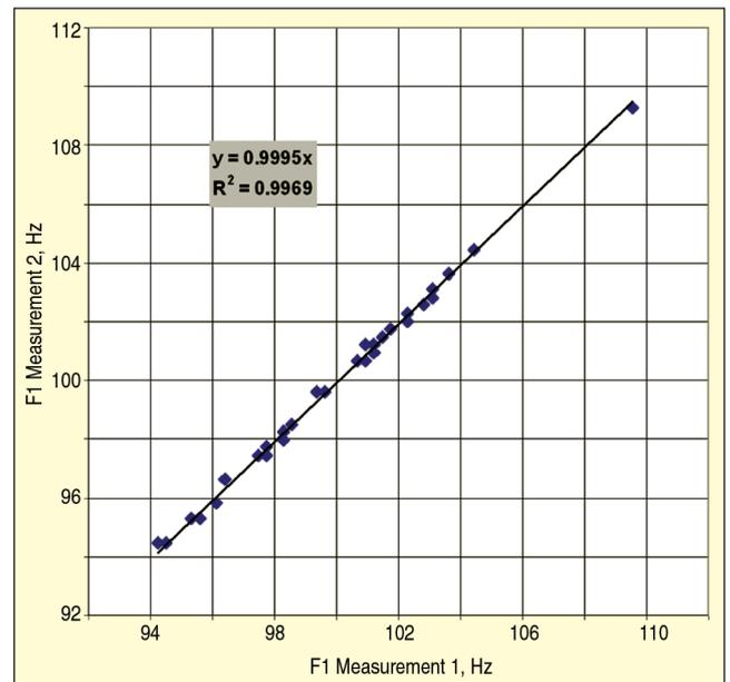
Figure 16. Isoplot from first natural frequencies.
