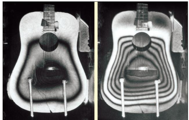
Figure 11. Time-averaged holograms of acoustic guitar top. (Courtesy Karl Stetson Associates LLC, [www.holo fringe.com](http://www.holo fringe.com).)
