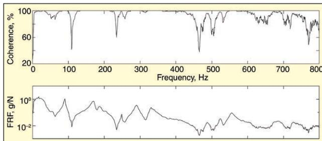
Figure 9. Typical FRF along with coherence and impact profile.
