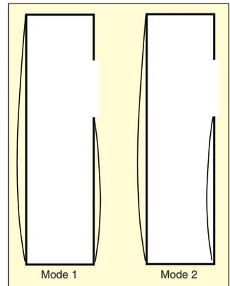
Figure 10. Lower modes of an acoustic guitar.
