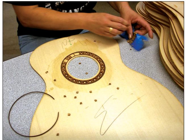
Figure 6. Applying sound-hole trim by hand.
