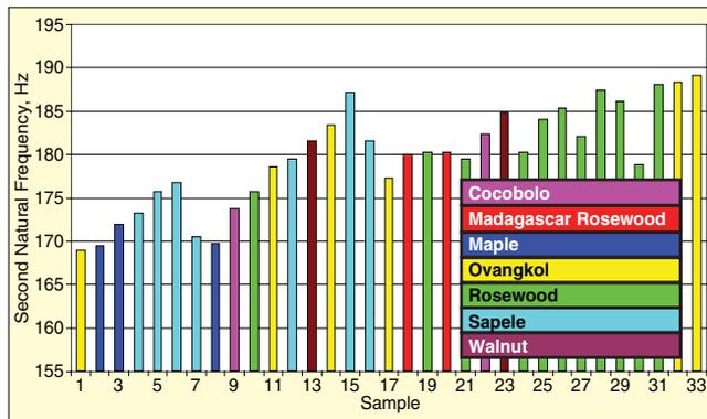
Figure 15. Second natural frequencies of instruments in test pool.
