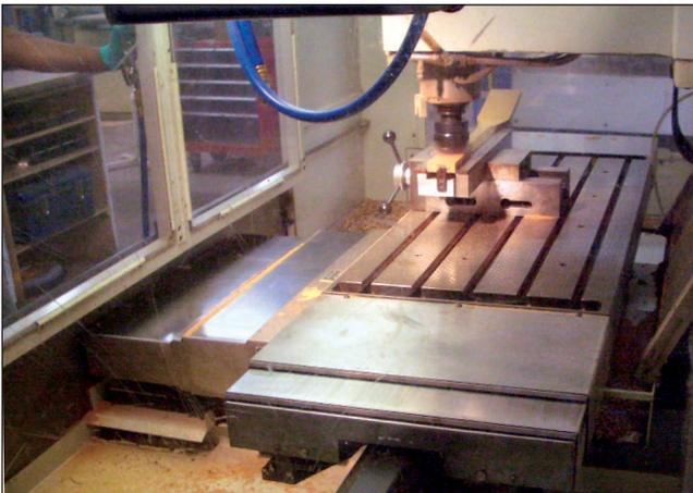
Figure 4. Machining a neck on large CNC mill.
