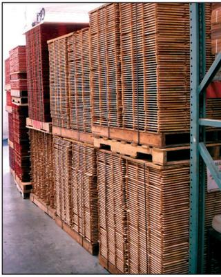
Figure 3. Stacked top and back blanks being conditioned before use.
