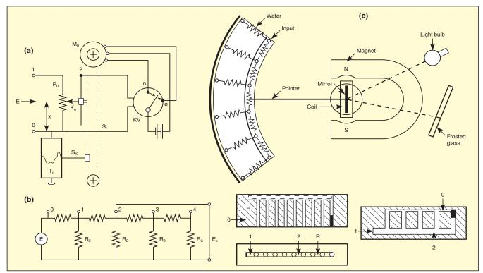
Figure 3. Jens Oskar Nielsen's logarithmic potentiometer is a chain of T-link resistors, where the resistive medium is water. (a) Principle of the writing logarithmic potentiometer. (b) Some of Nielsen's original drawings. (c) Practical construction of level recorder, with a moving coil element, and pointer tip that dips into the water potentiometer. Total dynamic range can be changed by changing the water level,
