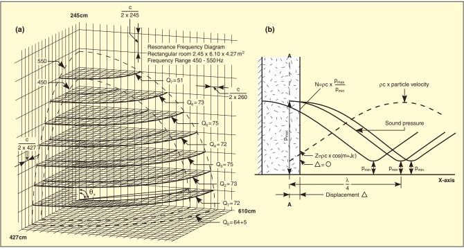
Figure 10. (a) Frequency of a standing wave in a rectangular room (distance from center) and the directivity. Rapid increase in numbers stems from increasing frequency. (b) Impact of standing wave on porous absorption material. From position at  $p_{min}$  and ratio  $p_{max}/p_{min}$ , complex acoustic impedance can be determined. Real impedance is found in Plane A-A.
