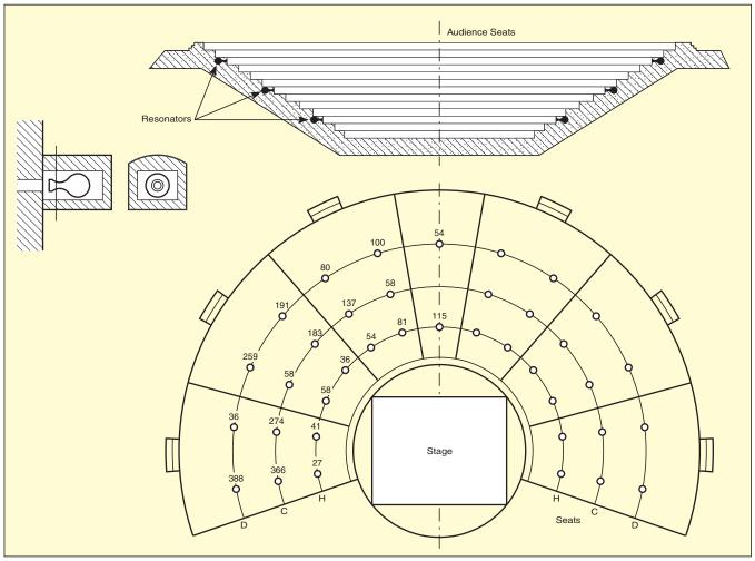
Figure 13. The drawing was made in accordance with what we think Vitruvius meant. Vases were situated under the seats with openings pointed to the center. Each vase was tuned to a different frequency according to a complicated procedure.
