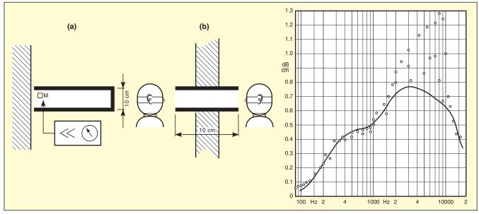
Figure 9. (a) P. O. Pederson's idea to measure the vibration amplitude of wall with a microphone in a tube lined with sound absorptive material. (b) 12-cm tube lined with sound absorptive material placed in a heavy wall. It was very difficult to communicate through the tube. Graph shows measured absorption. High attenuation at high frequencies makes speech difficult.
