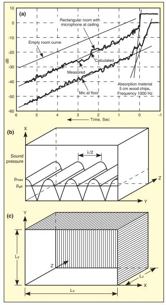
Figure 4. (a) Reverberation curves recorded with Nielsens's level recorder; note the detail. (b) Standing wave moving parallel to absorbing material covering the floor in a  $6 \times 6 \times 4$  m concrete room. (c) Only rectangular rooms, where each wall section has the same acoustic impedance, can be calculated by solving the wave equation.
