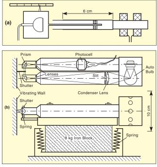
Figure 1. (a) Standing wave tube. (b) An optical instrument for measuring the vibration of a wall.
