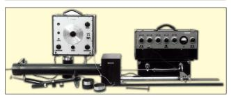
Figure 7. Beat-frequency oscillator (left) and line-powered frequency analyzer with two selective sections (six variable resistors and 8 × 6 fixed capacitors). Standing-wave tube (front). All were made at the army's workshop in Ryvangen in 1942 and were beautifully crafted.
