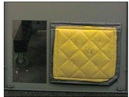
Figure 3. Blanket affixed to motor housing.
