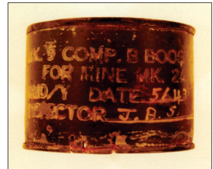
Figure 11. Small booster cap held enough explosive to set off the Torpex in a real submarine hit. Does anyone know "Inspector J.B.S. or the meaning of "NMD/Y"?"
