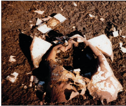
Figure 5. Remains of tail cone (propeller removed), which was corroded and damaged beyond repair. Note the two triangular-shaped rudders.
