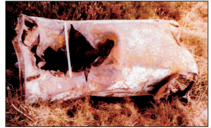
Figure 7. Torpedo body shell with hole inside after being unearthed and cleaned. The white line is a 12-inch-long hacksaw blade for size comparison.
