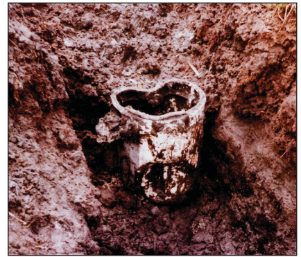
Figure 6. Torpedo body section found in 6 feet of earth. Tail cone was already removed. The torpedo had been in this acidic peat environment for about 40 years.
