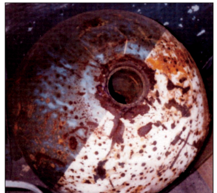
Figure 8. Torpedo nose section with fuse pocket in center after the fuse was carefully removed. Brian had been standing on the nose about 8 feet down while digging out the body section. After he got it out of the ground, he chopped away at some of the nose ‘ballast’ to make it light enough to pick up. He learned later that he had been chopping at ‘Torpex’ explosive. Marks on the detonator indicated that it had tried to detonate when it hit the ground, but the ‘soft’ landing in the peat probably didn’t provide a sharp enough impact to fully operate. The nose probably kept its shape because of the inside full of Torpex.
