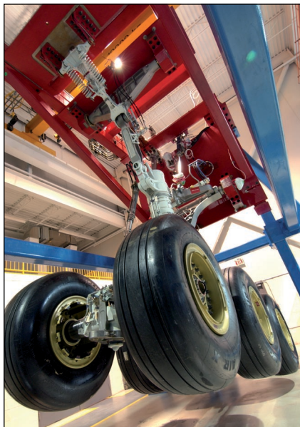
The six-wheel landing gear system weighs approximately 12,000 pounds and is more than 25 feet long when fully extended.
