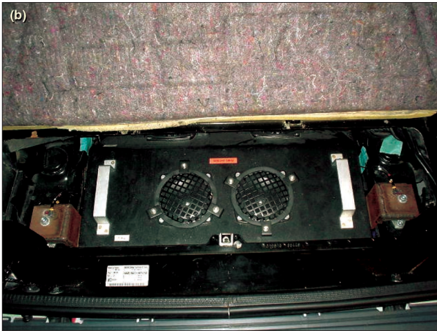
Figure 2. Engine noise and vibration simulator placed in vehicle.
