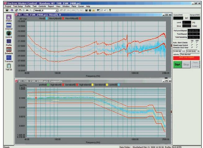
Figure 9. The same test automatically shut down by  $H^1$  limits when the fixture failed.
