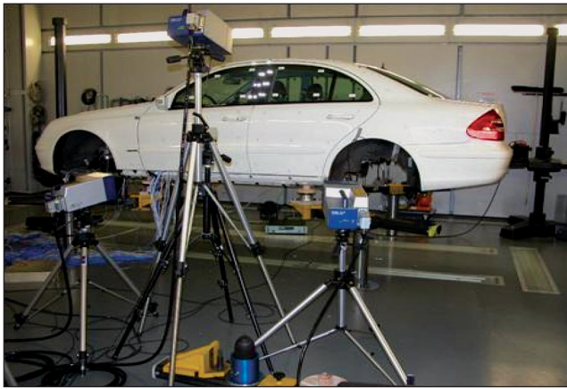
Figure 1. 3D-SDLV scan heads measuring a car body.
