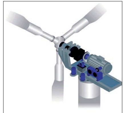
Figure 3. Wind turbine cutaway showing hydraulic actuators in place
